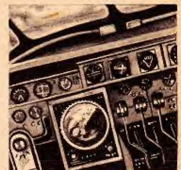
The radarscope in an aeroplane is used to detect storms and other disturbances in the air more than 100 miles away.
